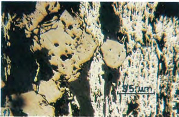
f) Granular magnetite showing banding (So) alternating with coarse specularite in a chertic matrix. Pedrada, D.D.H. S-11, 40 m.
