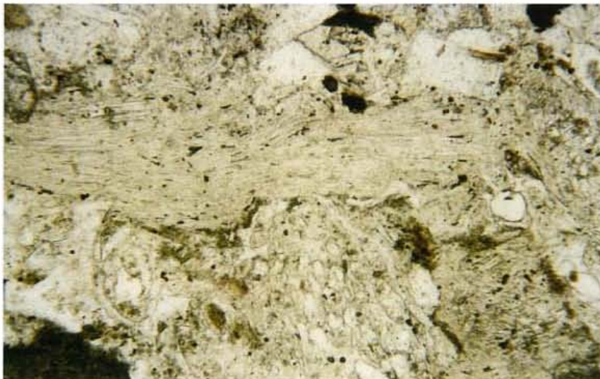
Fig. 6 — Some examples of pumice fibrous and spheroidal vesicles (photomicrograph take with parallel nicols).
