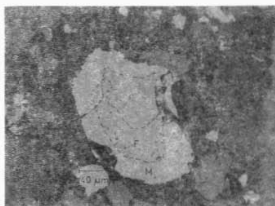
Fig. 2 — Irregular shaped core of aluminous chromian spinel (C) enveloped by ferritchromit (F) showing symplectic intergrowth plagioclase (dark grey) mantled by lighter titanomagnetite (M)
